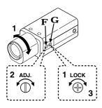
**F** Flange-back adjustment screw (FLANGE BACK ADJ.)
